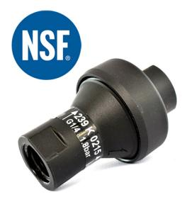
The pre-set EcoReg® fluid regulator is an independent diaphragm pressure regulator that can be installed in all fluid systems. The pressure regulator ensures a constant and precise output pressure independent from the input pressure. The pressure value has been factory preset and cannot be changed. This ensures that no one can manipulate the specified pressure value.
